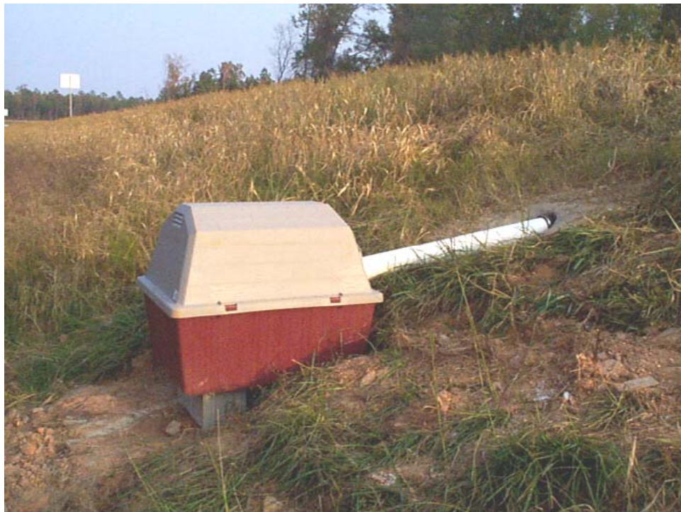
Photo 28. Doghouse enclosure for a tipping bucket
