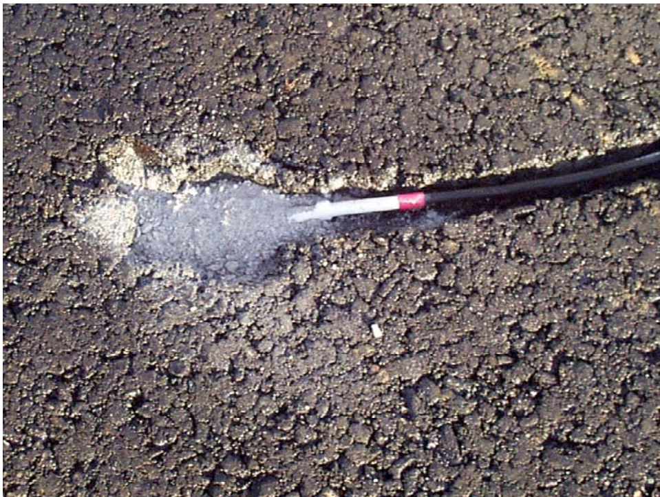
Photo 20. Thermistor protected with fine aggregate
