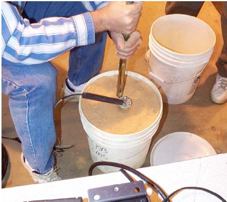
Photo 9. Calibration of the Sentry 200 moisture probes
