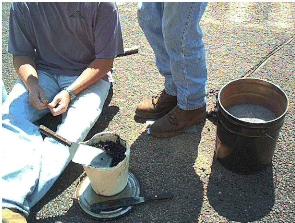
Photo 24. Stepping on a metal plate to compact hot-mix over the probe at the pavement surface
