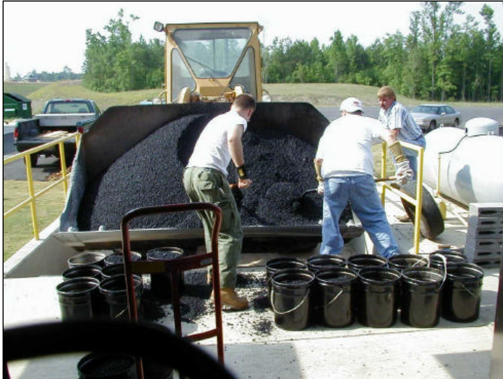
Figure 26. Sampling for Performance Test Specimen and Bulk Storage Purposes.
