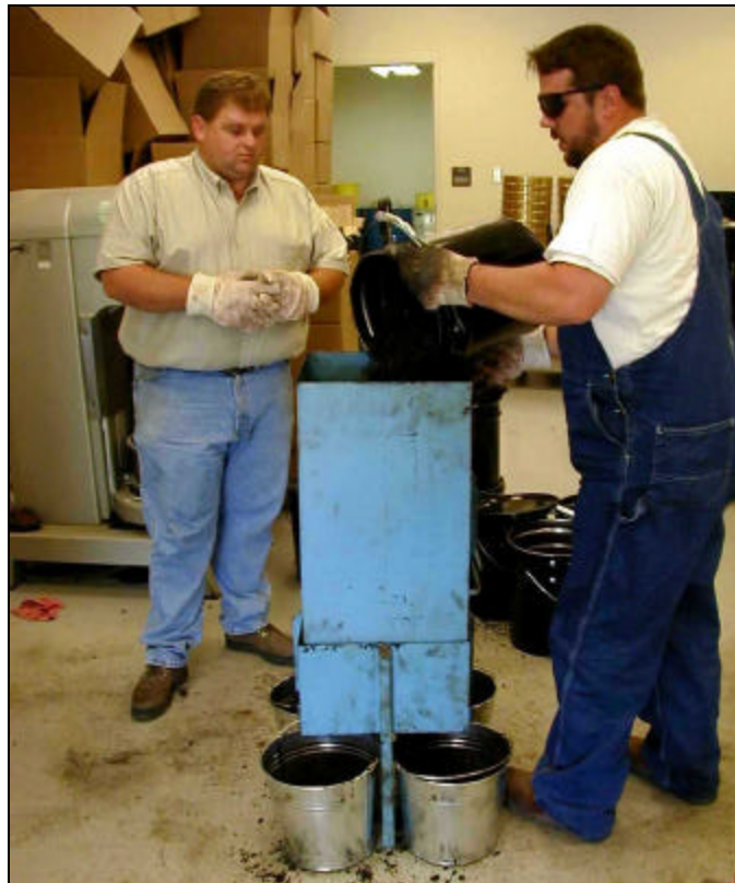
Figure 24. Splitting with the Gilson Quartermaster.
