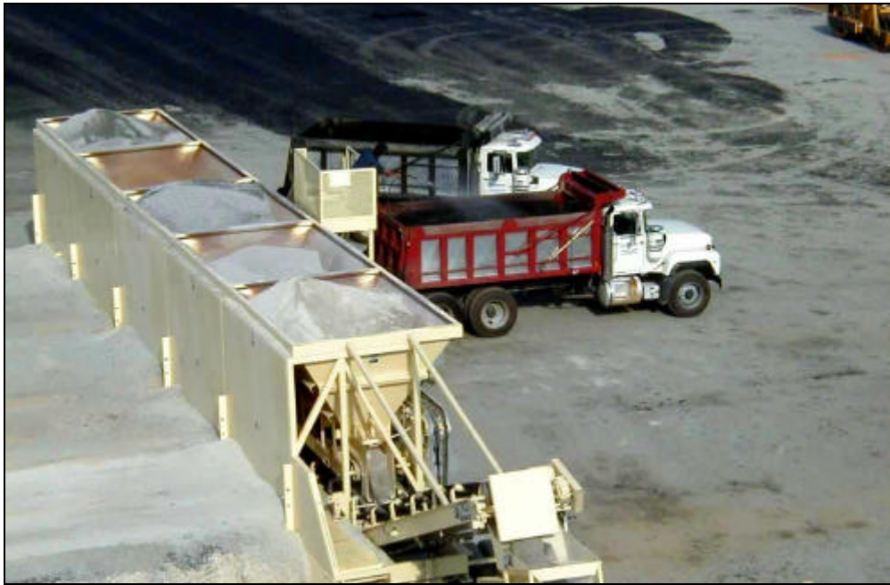
Figure 13. Truck Beds Being Spraying with SPX-7 Release Agent.
