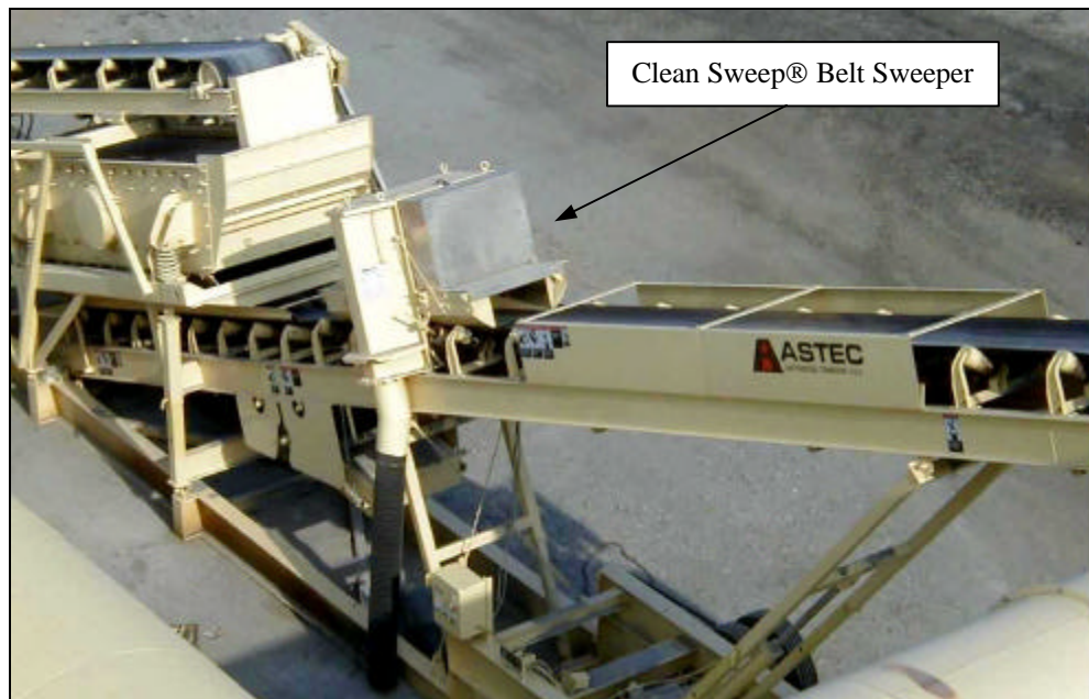
Figure 12. Mechanical Coldfeed Sampling Device.
