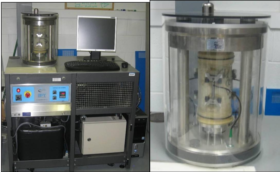
**FIGURE 6.11 The AMPT Machine and Close Up of Specimen.**
