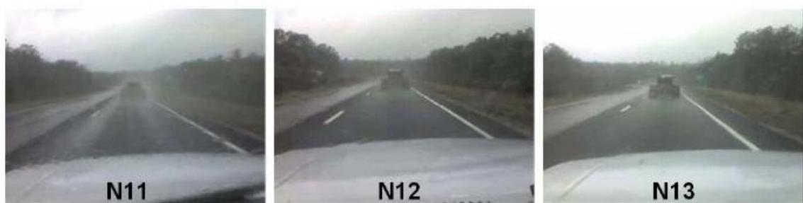
**FIGURE 3.25 Road Spray Observed Following Four Hours (6 mm per hour) of Rain During Fleet Operations (14).**
