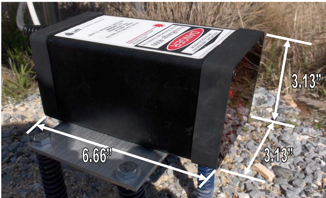
Figure 3.15 AR4000-LIR Distance Measuring Unit.
