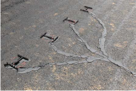
a. Gauges Laid Out with Sand Asphalt Tack under Gauges and Covering cables.
