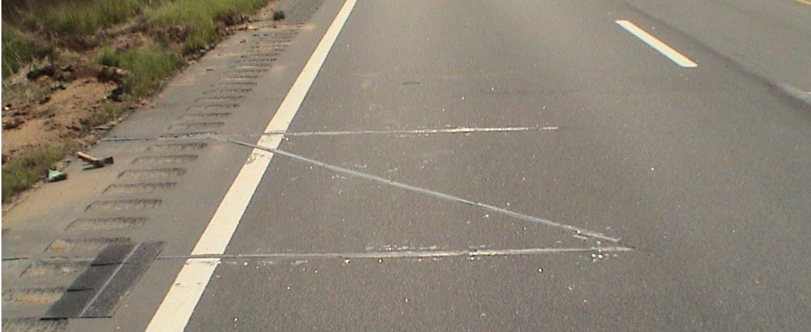
Figure 3.14 Axle Sensing Strips for Measuring Wheel Wander.
