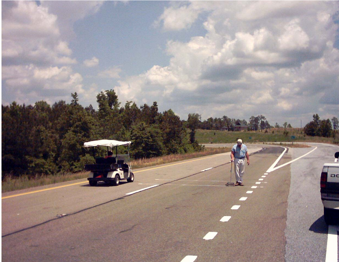
Figure 3.3 Rutting Measurements with Dipstick.
