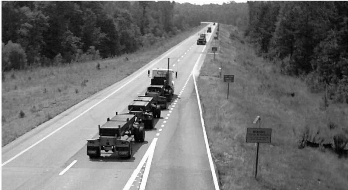
Figure 2.4 Triple Trailer Trains Used to Apply Accelerated Loading.
