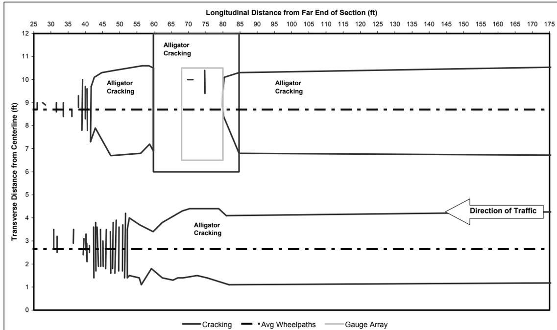
**Figure 5.24 N2 Crack Map 10/18/2004.**
