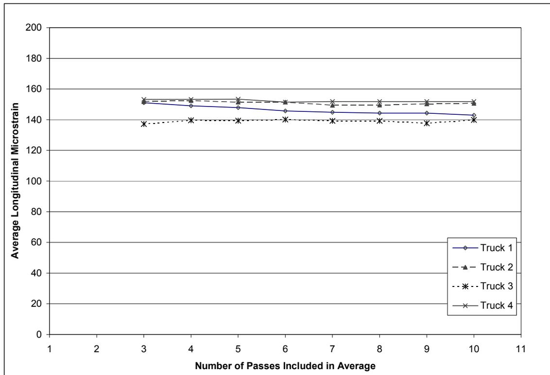
Figure 5.6 Average Strain by Truck and Pass.
