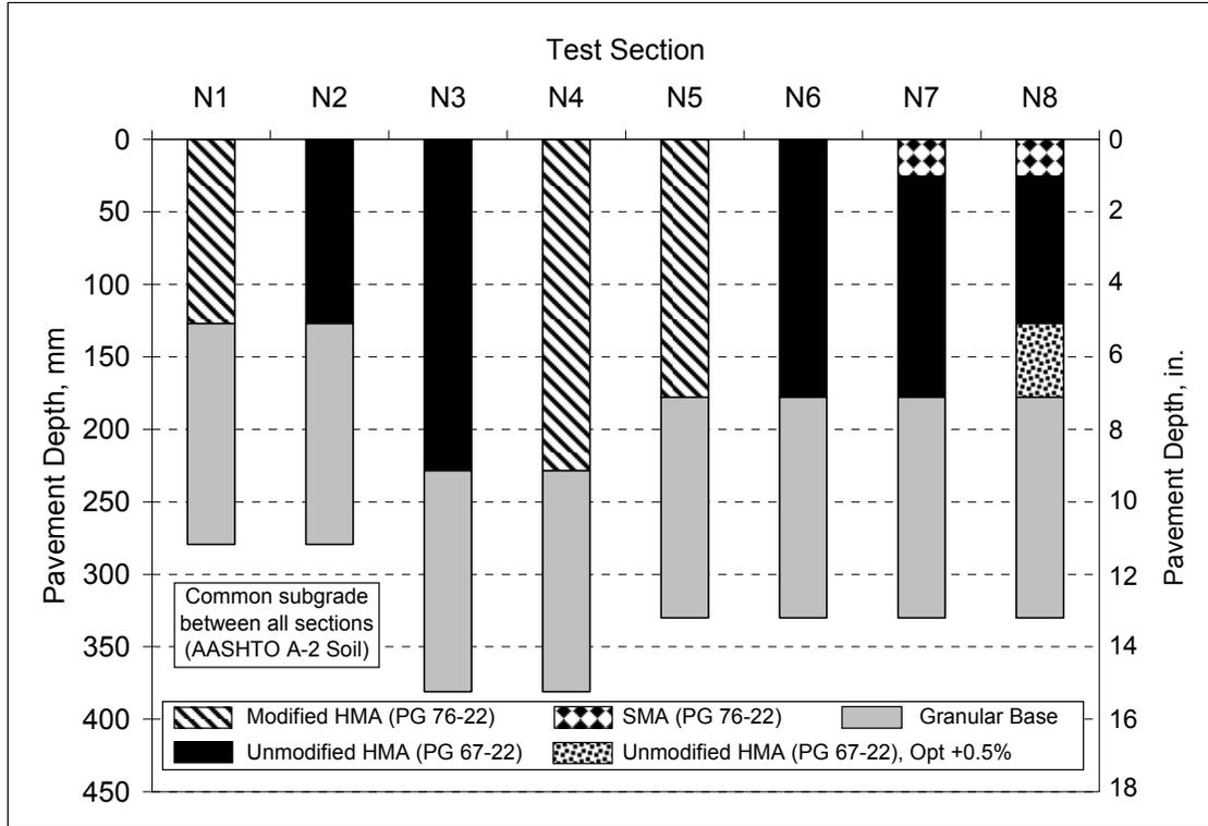
Figure 1.3 Test Section Layout.
