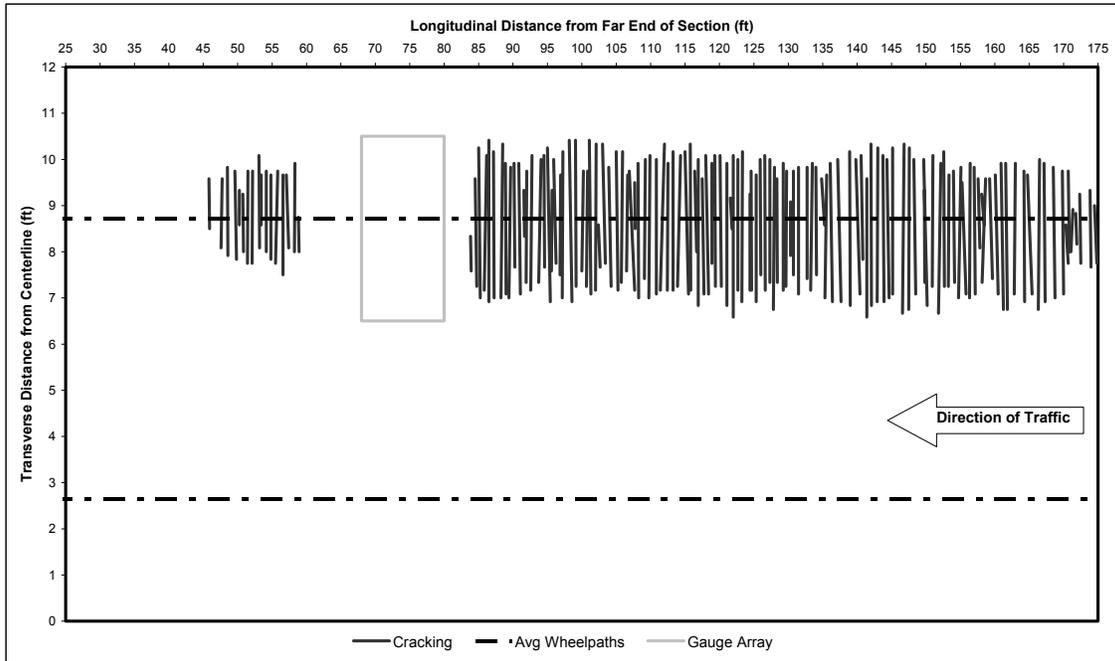
Figure 5.22 N2 Crack Map 6/28/2004.
