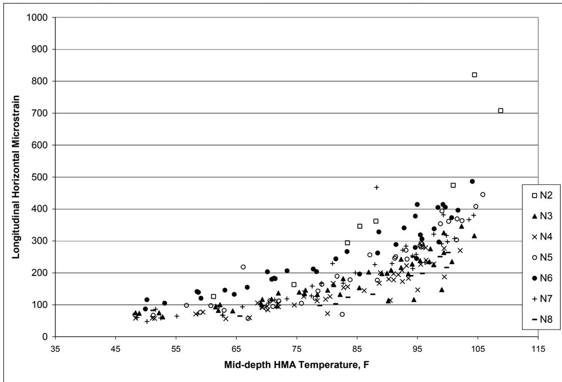
Figure 5.15 Box Trailer Strain – Temperature Relationship.
