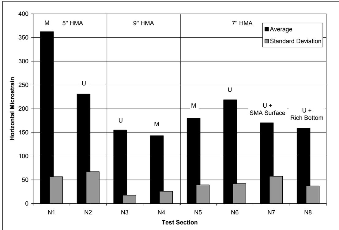
**Figure 5.13 Temperature-corrected Strain Data by Test Section.**
