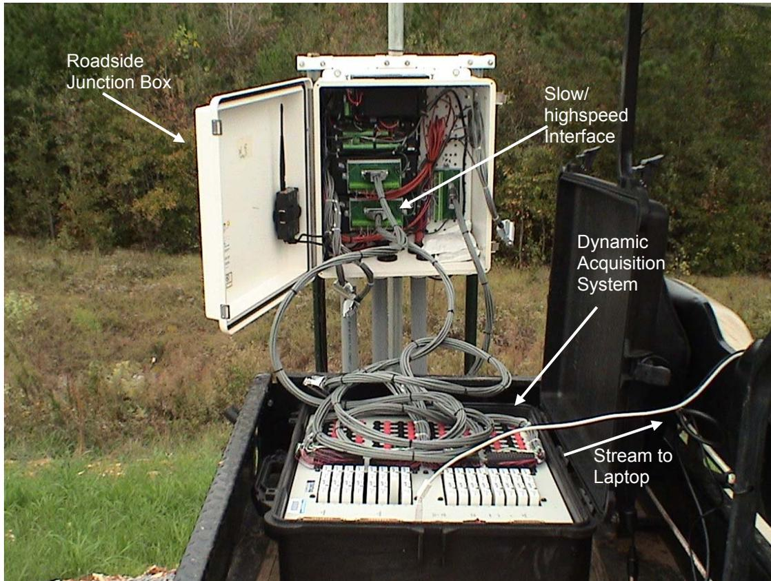
**Figure 3.7 Dynamic Data Acquisition Scheme (Timm et al., 2004).**
