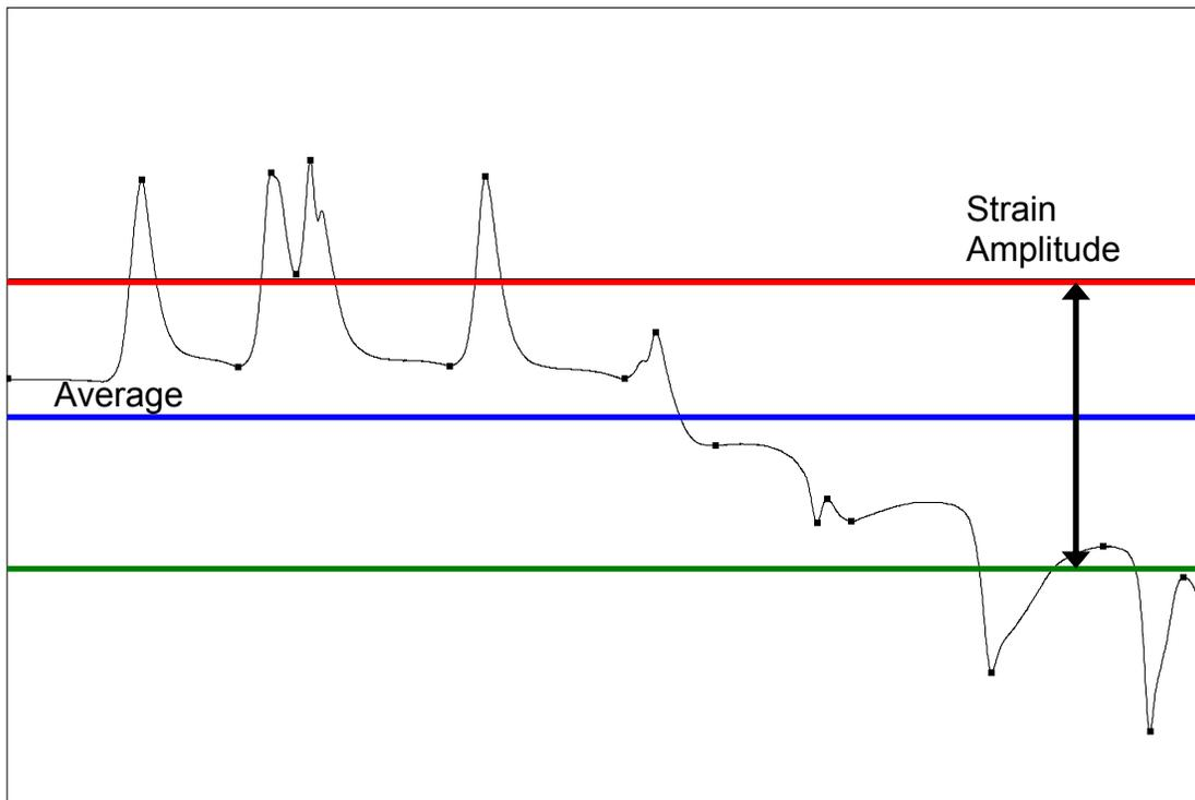
**Figure 4.8 Strain Amplitude Illustration – Example 2.**
