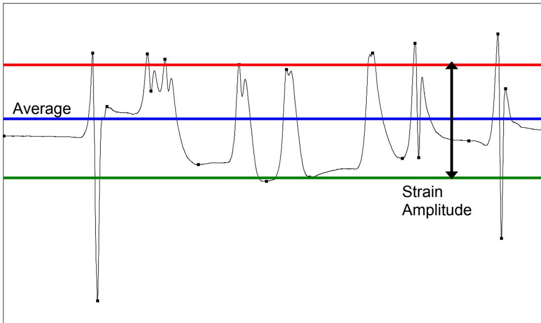
**Figure 4.9 Strain Amplitude Illustration – Example 3.**
