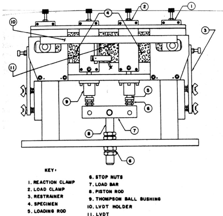
Figure 2.5 Schematic of Third Point Beam Fatigue Test (Monismith et al., 1985).
