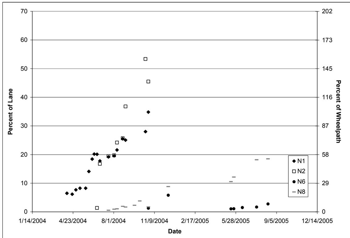
Figure 5.25 Percent Fatigue Cracking by Date.
