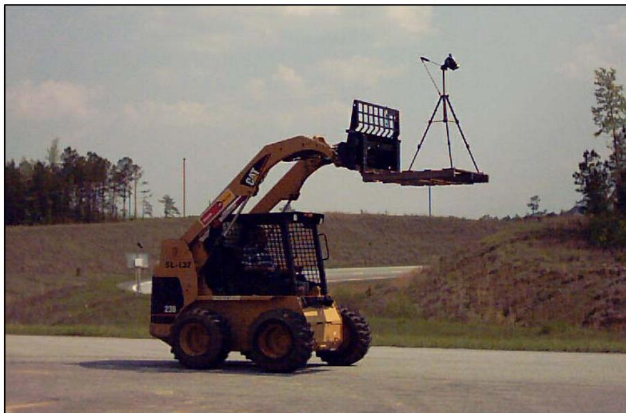
Figure 3.10 Camera Apparatus for Crack Record.
