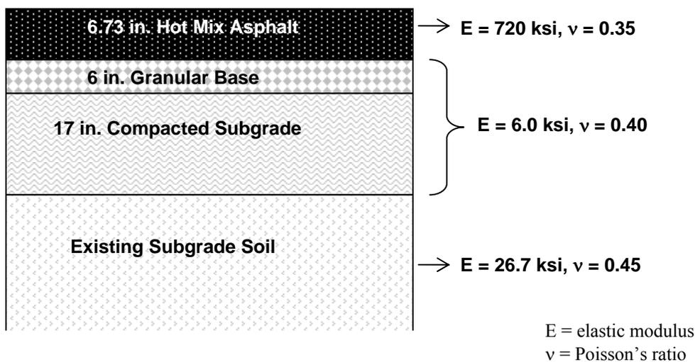
**Figure 4. Cross Section of Test Section N5.**
