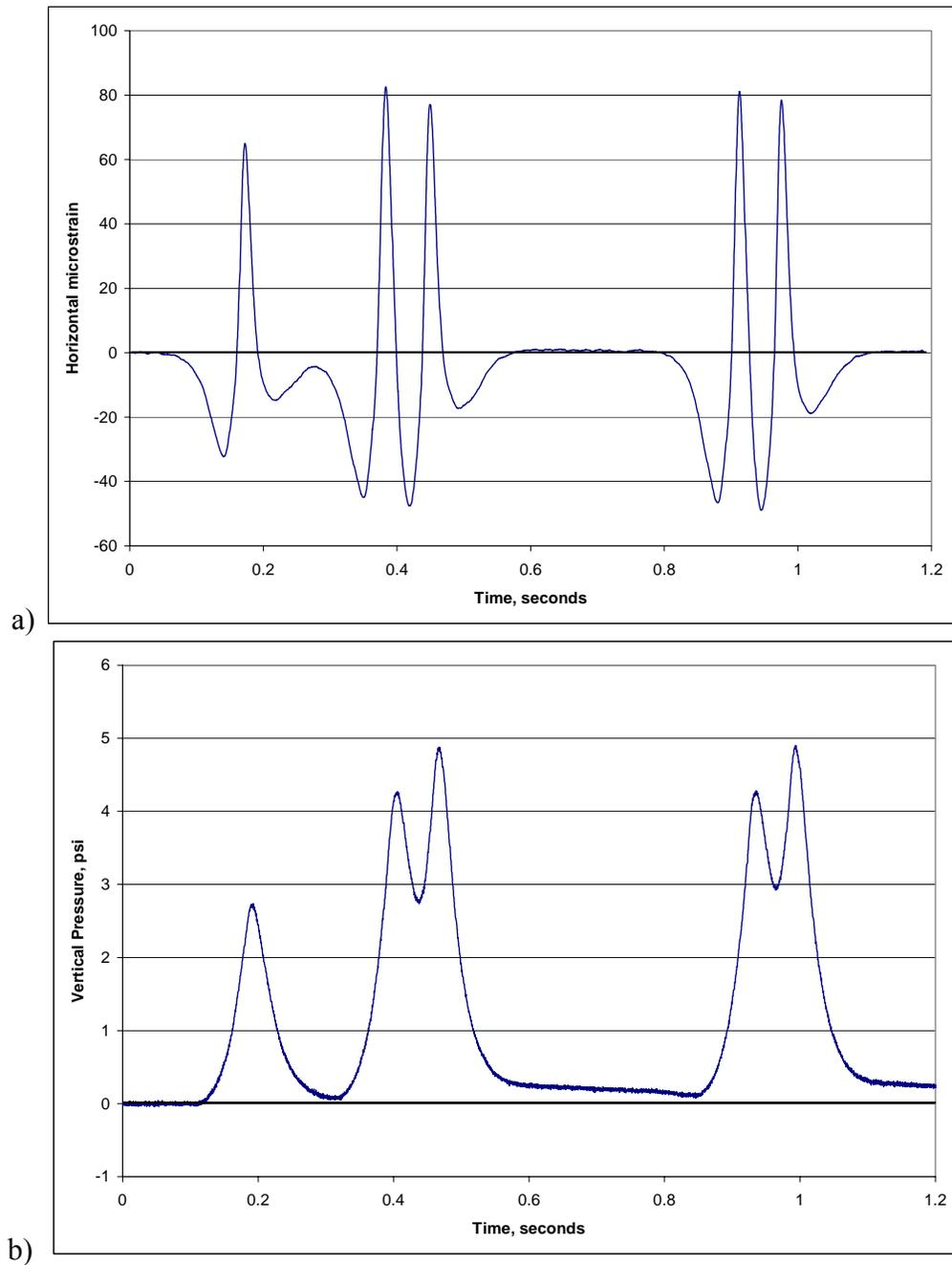
**Figure 14. Dynamic Pavement Response a) Strain b) Pressure.**
