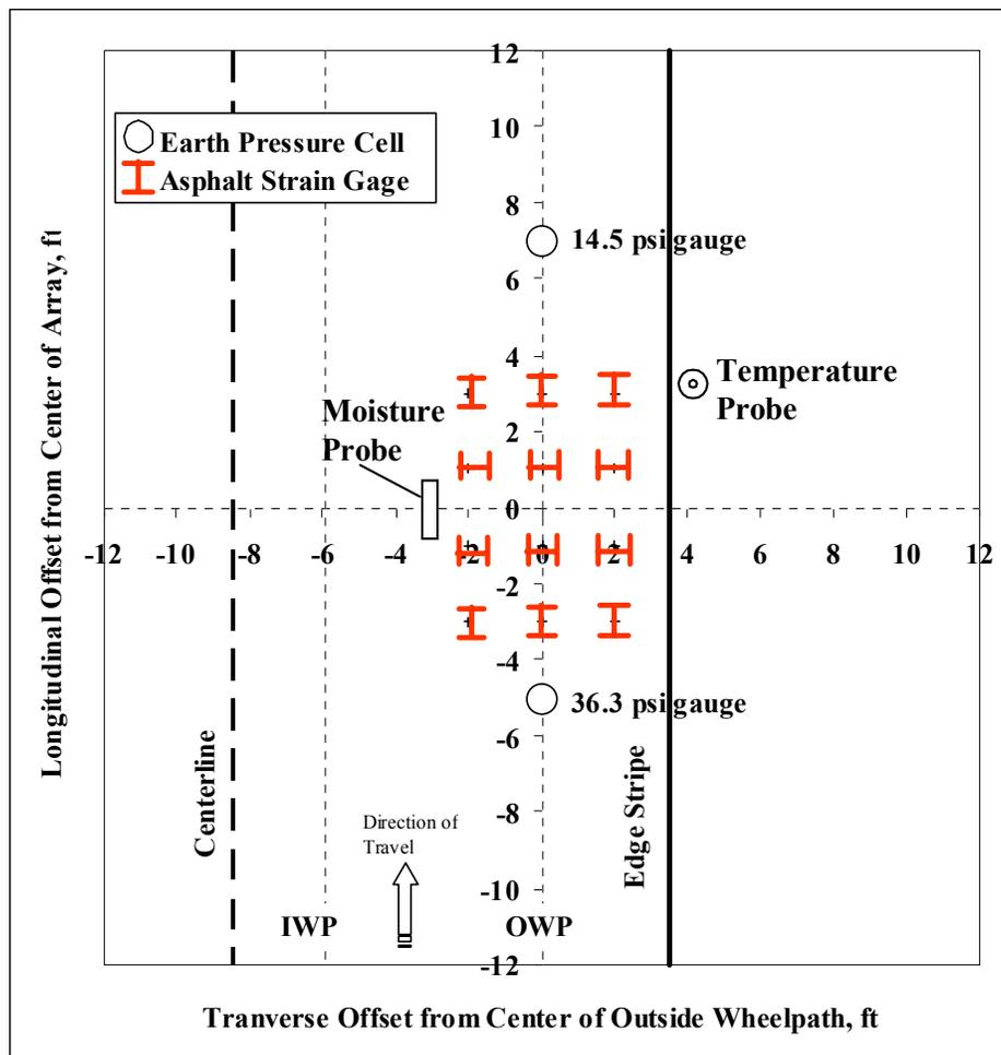
Figure 9. Instrumentation Schematic.
