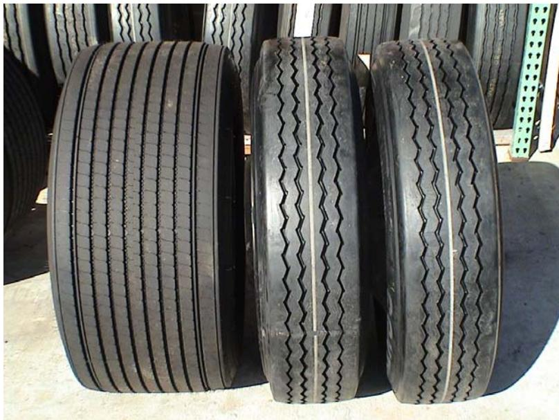
**Figure 2. Wide-Base Single (445/50R22.5) and Standard Dual (275/80R22.5) Tires.**
