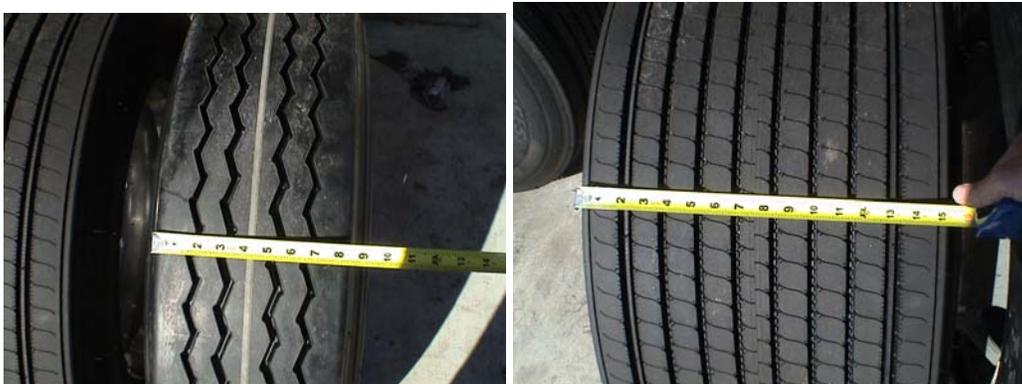
**Figure 1. Standard Dual Tire and Wide-base Single Tire.**
