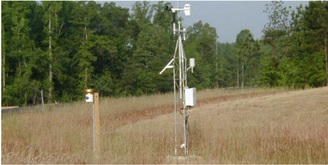
Figure 37 – Automated Weather Station (Structural Study in Background)
