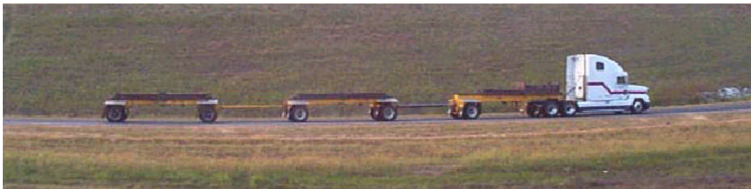
Figure 33 – Triple Trailer Trains Used to Apply Accelerated Loading
