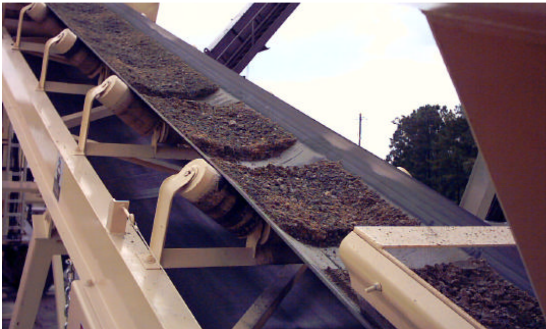
Figure 8 – Recovering Random Sample Portions from Cold Feed Belt at Plant
