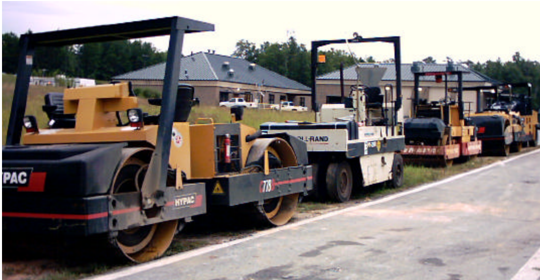
Figure 10 – Fleet of Rollers Utilized to Achieve Density on Track
