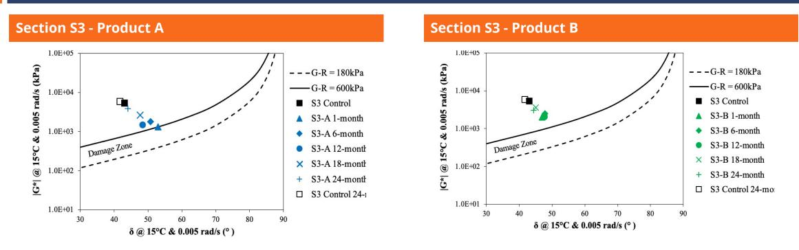
□ S3 control binders (1- and 24-month field aging) located above the *G*-*R* 600 kPa limit.
