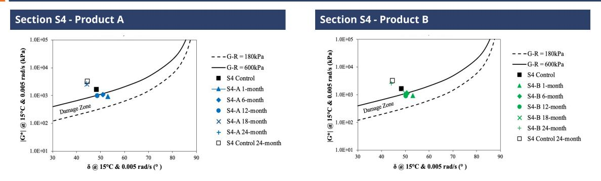
□ S4 control binders (1- and 24-month field aging) located above the *G*-*R* 600 kPa limit.
