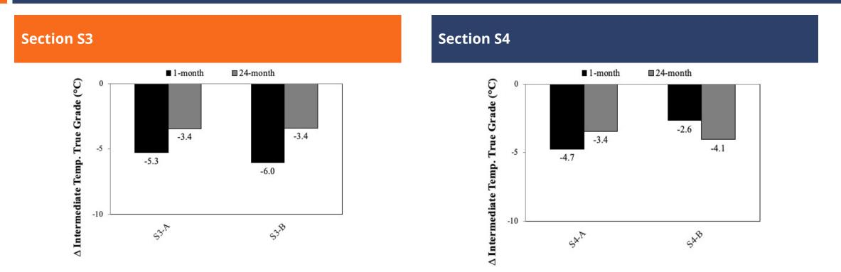
A decrease in the intermediate pass/fail temperature of control binders was observed after treatment application, increasing the fatigue resistance of control binders.
