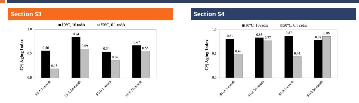
□ All spray-on rejuvenator products showed |G\*| aging index below 1.0 after 1 month and 24 month of application, indicating that the stiffness of the binders extracted from the treated sections remained below the stiffness of the control binders measured after 1 month and 24 month of field aging.
