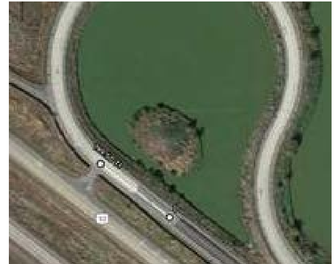
OGFC/PCC conventional tack OGFC/PCC ultrafuse tack
