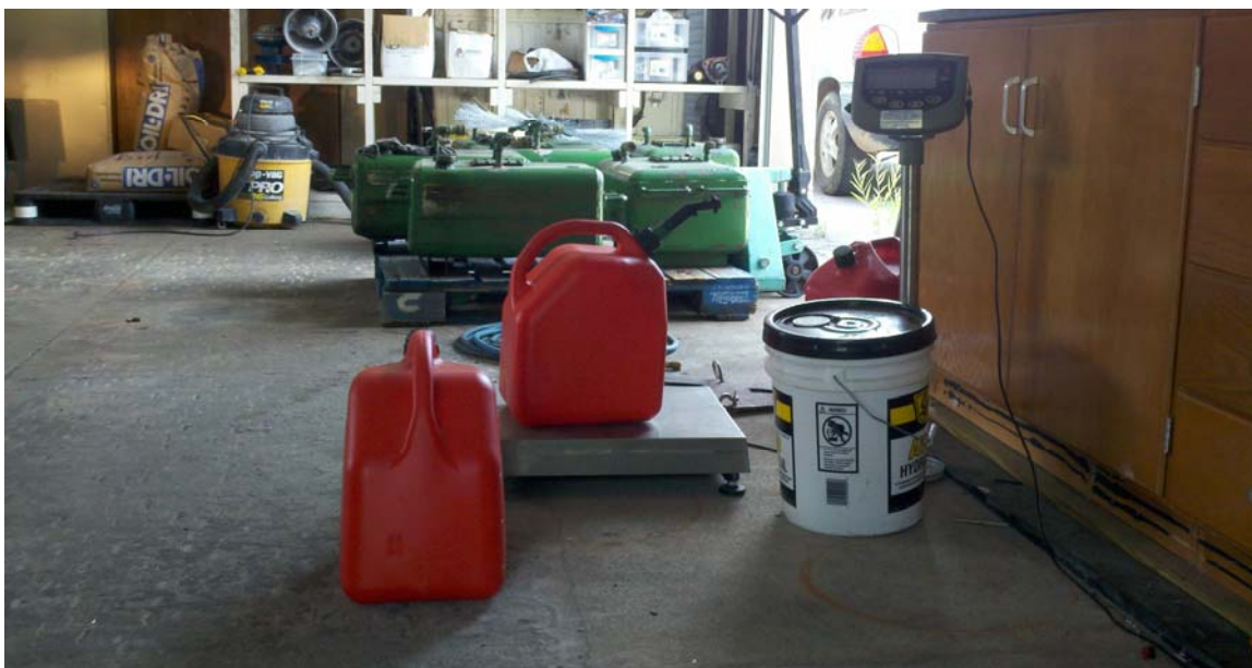
Figure 7 – Gravimetric Measurement of Fuel Consumption
