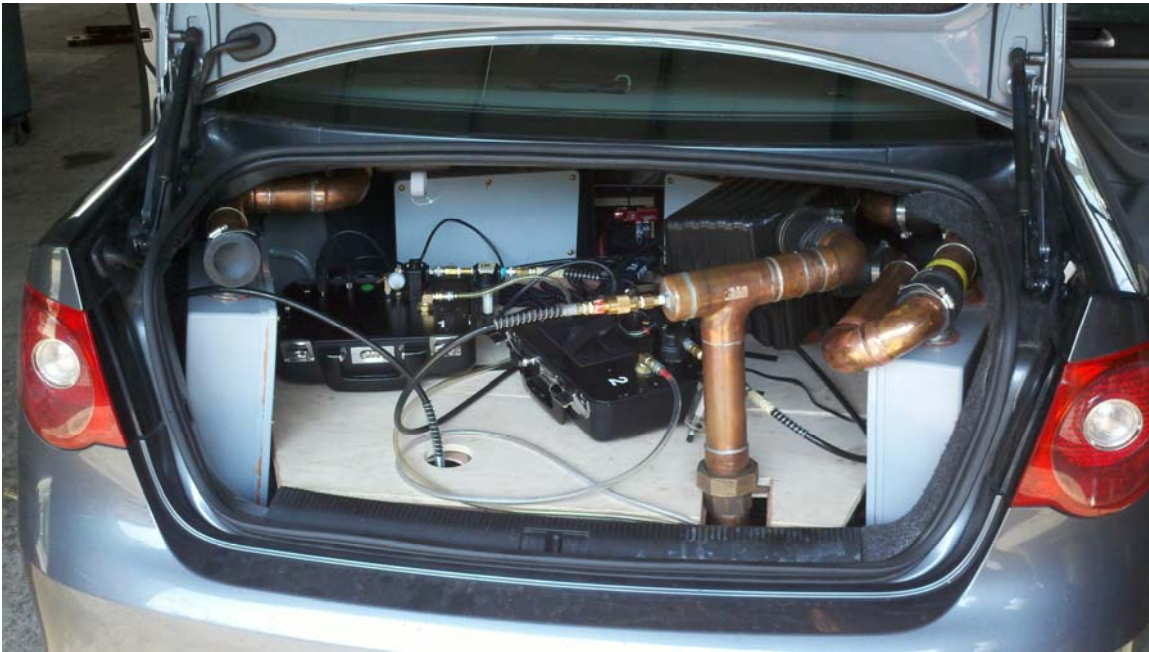
Figure 2 – Prototype Strataclear™ CO 2 Reducer System Installed in Trunk
