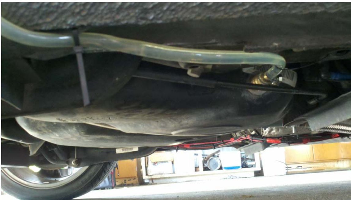
Figure 5 – Sight Tube Installed in Fuel Tank to Measure Volume of Fuel Consumed
