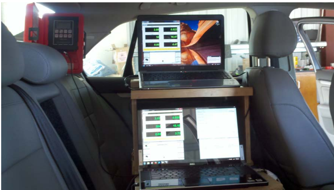
Figure 3 – Onboard OBD-II and Emission Monitoring Computers
