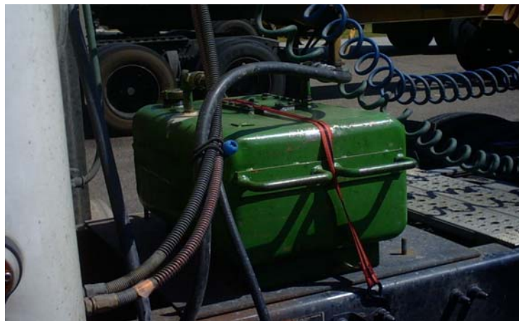
Figure 3 – Portable Fuel Tank
