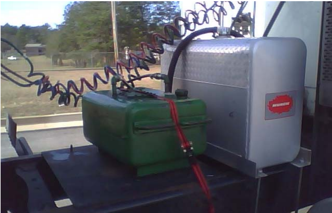
Figure 3 –Portable Weigh Tank
