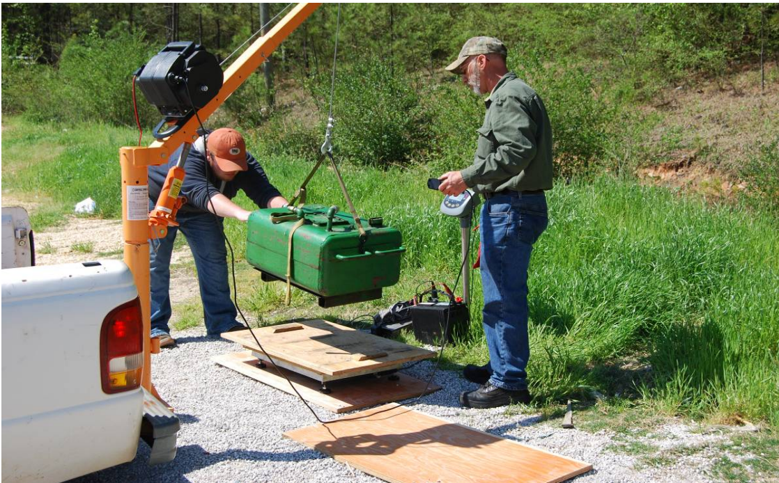
Figure 4 – Weighing Portable Tank to Within a Tenth of a Pound
